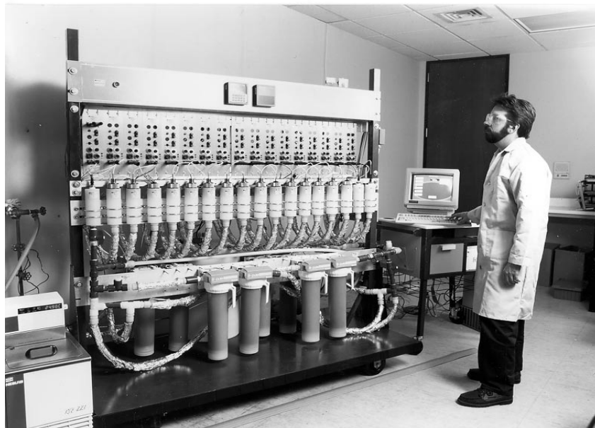
Figure 2 - Cell Constant Calibration/Certification System (Thornton Inc.)
